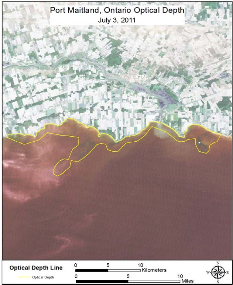
Figure 6: Recent water clarity/optical depth, derived from Landsat 5, extent analysis area near Port Maitland, Ontario Lake Erie. July 3, 2011
